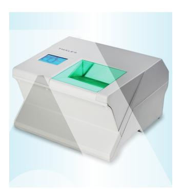
The Cogent Palm Scanner MultiScan527 is the definitive livescan for law enforcement applications. Offering superior image quality and matchless acquisition speed the Cogent Palm Scanner MultiScan527 acquires not only 10-prints, rolls and half-palms but also all types of supplemental prints as per fbi standards: thenar (ball of palm), full finger (distal, medial and proximal) and fingertip impressions.
